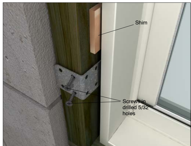
Figure 7: Attaching window with structural brackets.
