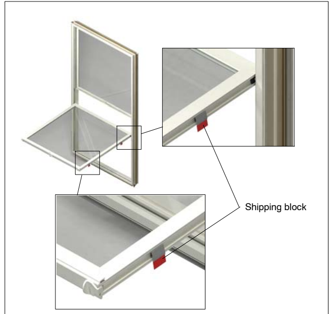
Figure 12: Double Hung unit shipping block removal.
