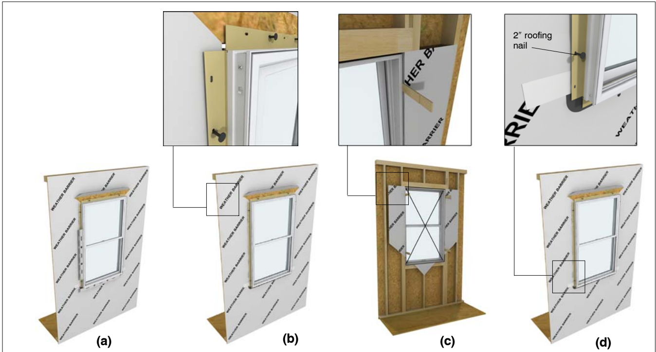
Figure 6: Positioning the window in the opening
