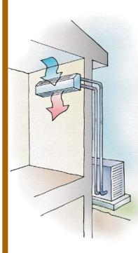
heating efficiency significantly. Some ductless minisplits can now be used for heating in very cold climates.
